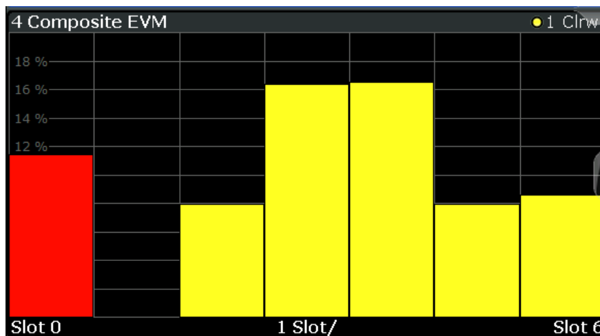
Figure 3-5: Composite EVM display for TD-SCDMA BTS measurements
