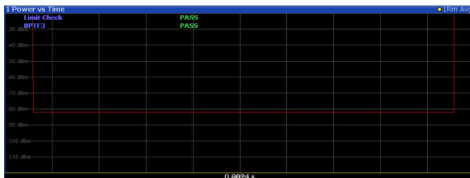
Figure 3-16: Power vs Time diagram for TD-SCDMA BTS application
